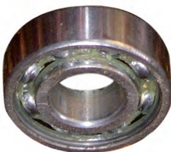
Fig. 12.16 : Ball bearings reduce friction
